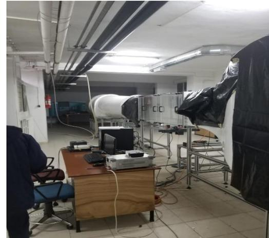
Figure 3. Wind tunnel main view (Erciyes University Faculty of Aeronautics and Astronautics Aerodynamics Laboratory)
