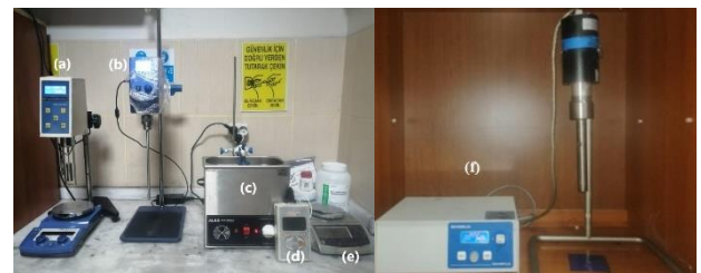
Fig. 2. Nanofluid preparation and property measurement setup
