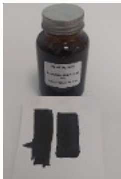
Fig 6- Electrode slurry and its visual testing on paper.
