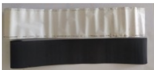
Fig. 2 - Disassembled standard commercial supercapacitor
