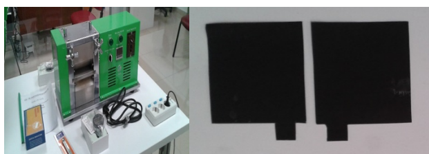
Fig. 8 - Hot roll press machine (TOB-JS100L) and prepared electrode.
