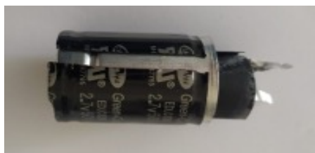
Fig. 2 - Disassembled standard commercial supercapacitor
