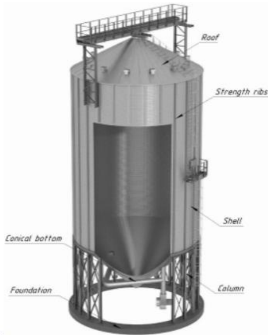
Fig. 6. Elevated (conical bottom) and above ground (flat bottom) silos: a) above ground (flat bottom silo), b) elevated (conical bottom silo) [49].
