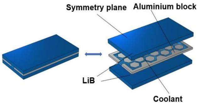
**Fig. 10.** Honeycomb Shaped Mini Channel Cold Plate [20]
