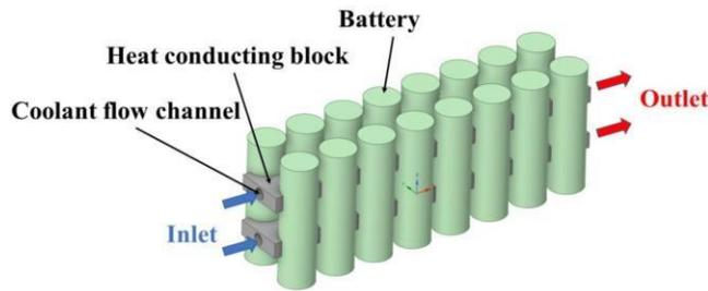
Fig. 7. Air and Liquid Cooling HCB [17]
