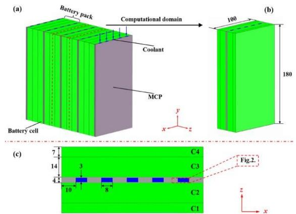
**Fig. 11.** Pin-fin Added Mini Channel Cold Plate [21]
