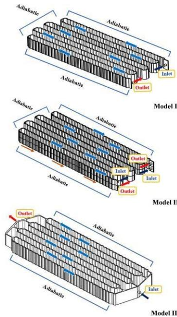
**Fig. 2.** Serpentine Mini Channel for 444 Cylindrical LiBs [12]
