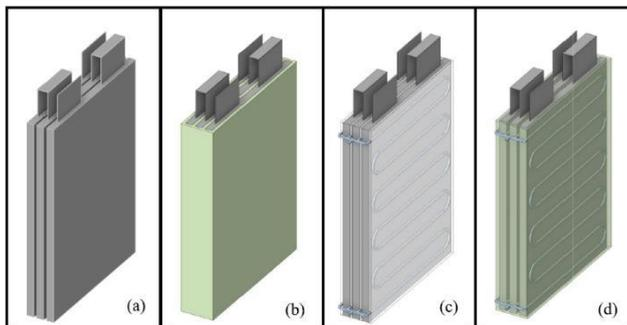
Fig. 8. PCM and Serpentine Mini Channel Cooling [18]
