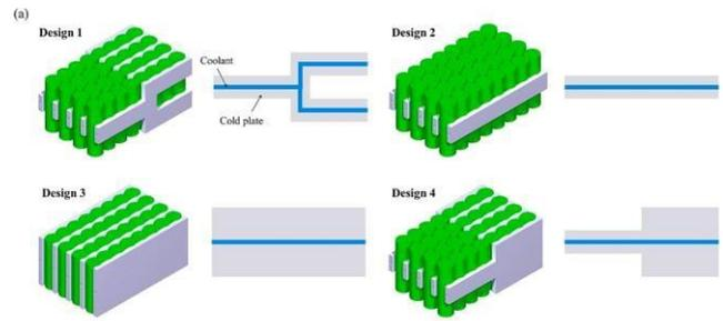
**Fig. 3.** Wrench Shaped Mini Channel Cold Plate [13]
