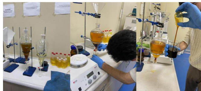
Fig.12 Sedimentation Process (in the separatory funnel)
