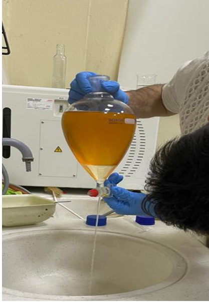
Fig.13 Washing Biodiesel with Pure Water
