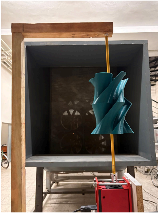
Fig. 8. Model 5 - The experimental view of the hybrid/optimized blade models in front of the wind turbine
