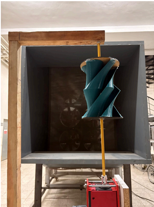
Fig. 9. Model 6 - The experimental view of the hybrid/optimized blade models in front of the wind turbine
