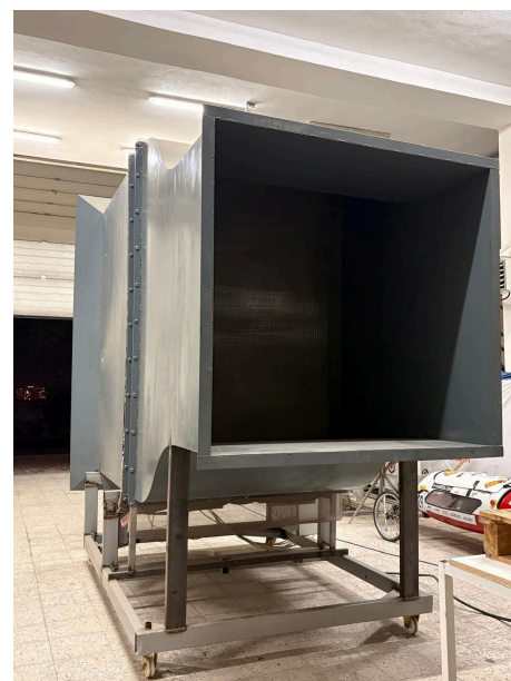
Fig. 2. The Wind Tunnel Used in The Experiment-2
