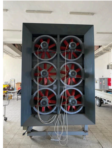
Fig. 1. The Wind Tunnel Used in The Experiment-1
