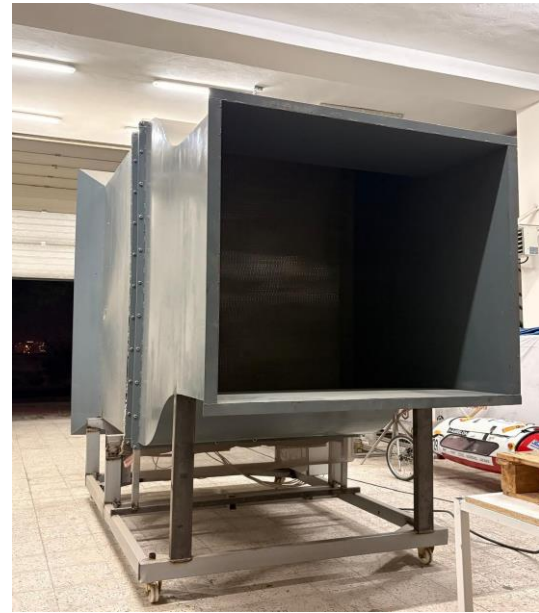
Fig. 2. The Wind Tunnel Used in The Experiment-2
