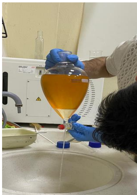
Fig.13 Washing Biodiesel with Pure Water
