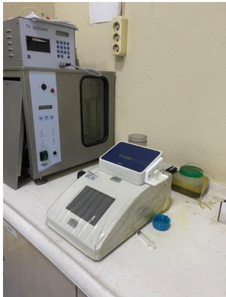
Fig. 2 Density Measuring Device – Krüss Optronic (Germany)
