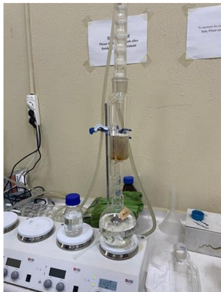
Fig. 6 Heated Magnetic Stirrer – DLAB MS-H340-S4
