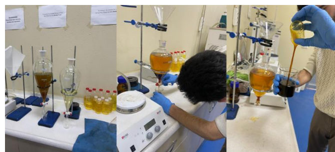
Fig.12 Sedimentation Process (in the separatory funnel)
